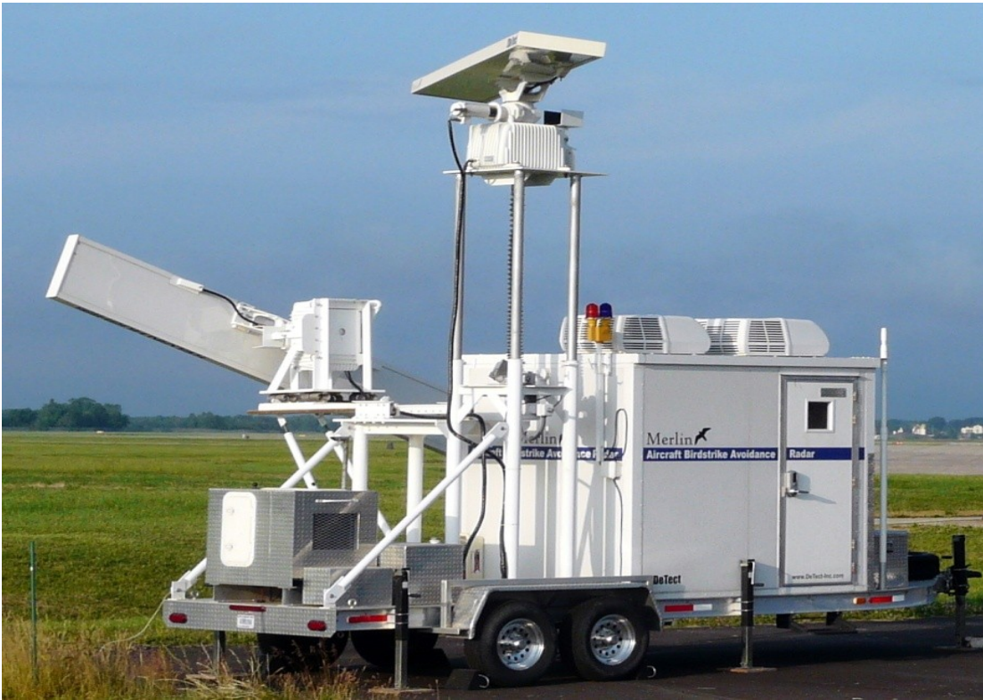
Figure 1. Merlin Avian Radar System at the Terre Haute International Airport.
