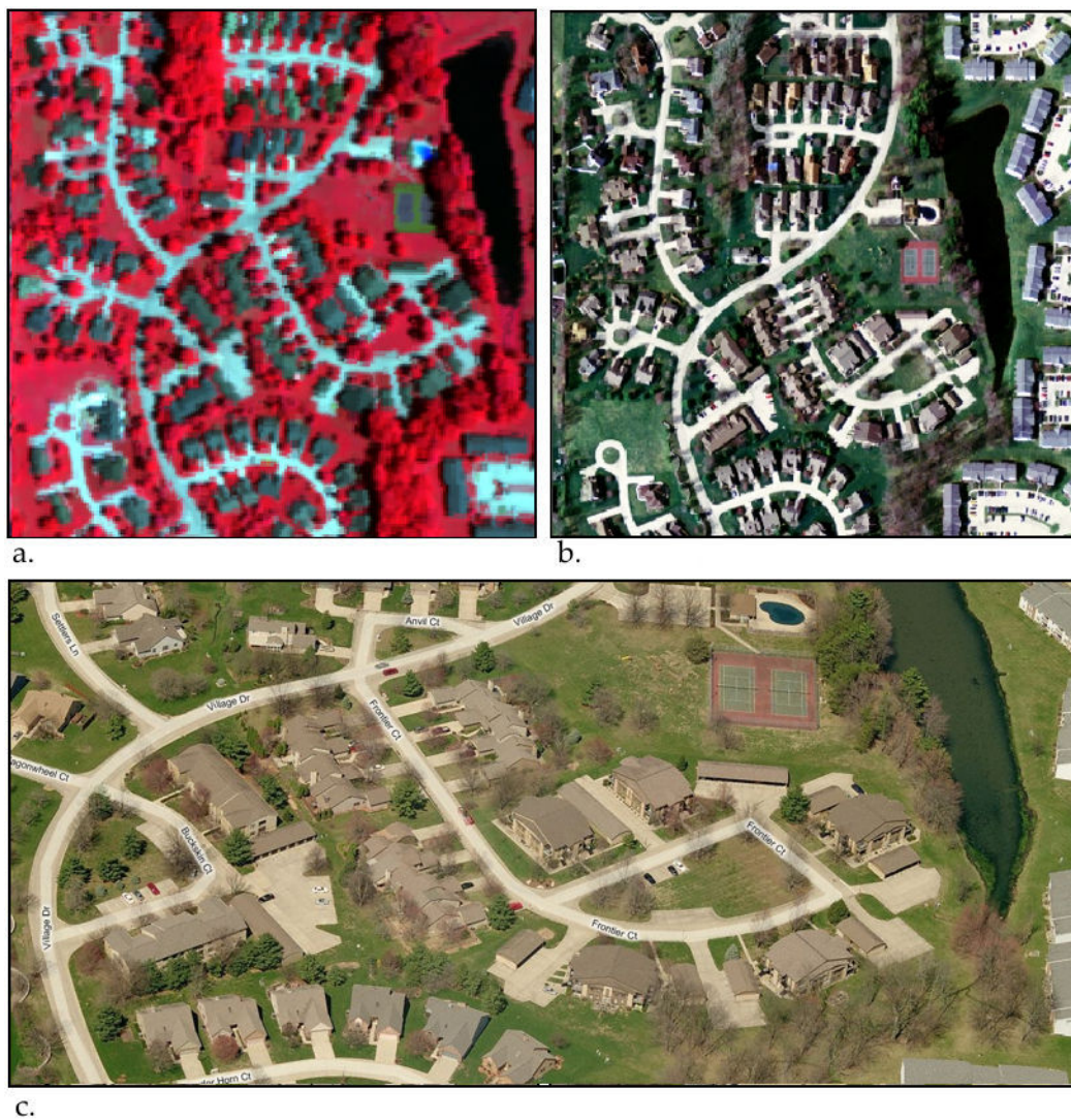
Figure 13. Subset of a residential area (2) with spatially less dense composition (See 4 in Figure 9): a. AISA+ composite of (RGB 187, 125, 63); b. DOQ; c. High resolution oblique aerial view of a part of subset.
