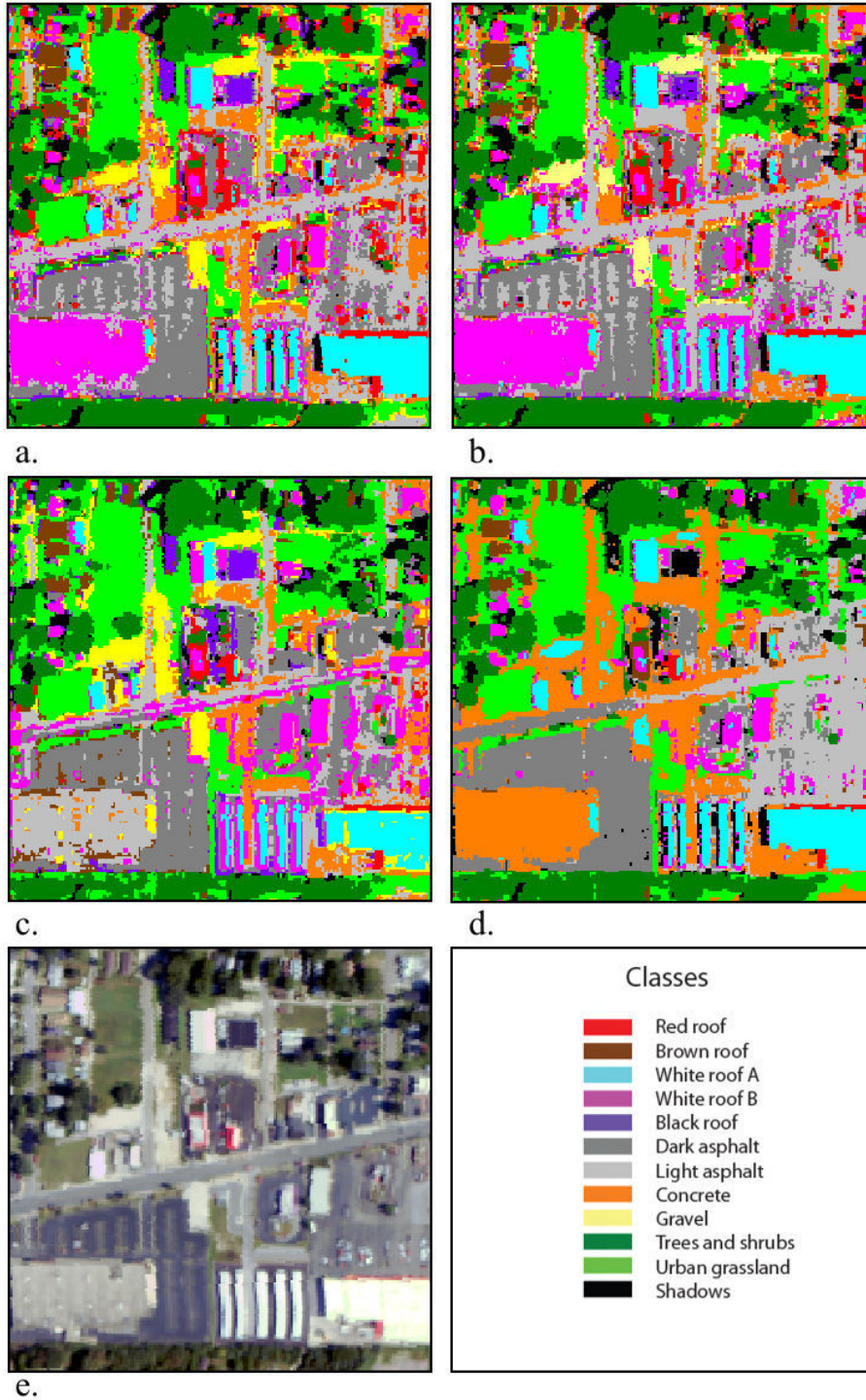
Figure 27. Classification results of commercial area (2) with a. MLC, b. ECHO, c. SAM, d. ISODATA, and e. Original AISA+ data are displayed in true color (RGB 135, 75, 25).
