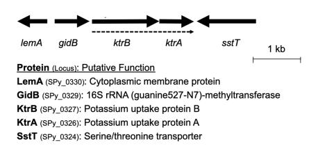
*Note.* Each arrow indicates an individual open reading frame and its orientation. *ktrB* is coexpressed with the downstream gene *ktrA*, which is shown with a dotted arrow under the *ktrB* and *ktrA* genes. The predicted proteins encoded by these open reading frames and their putative functions are shown below the gene organization.
