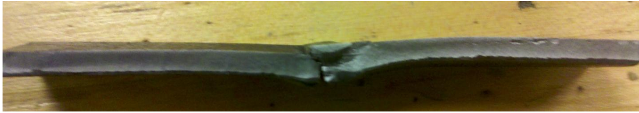
Figure 21. Cracking at weld joint due to shearing process.
